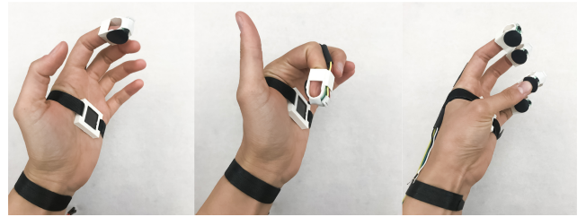
(b) Fingertip sensor and a magnet module can be seen in the first image (i); as the finger is bent and approaches the magnet, the hall effect sensor changes state (ii); the FSR sensors output continuous data to control frequency, gain, and filter and effect parameters (iii).
