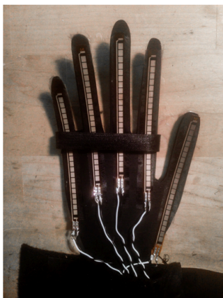
Figure 3. a.) Hand skeleton, b.) Outer layer with string attachments, c.) Inner layer of the armband showing the circuit board and sensor connections.
